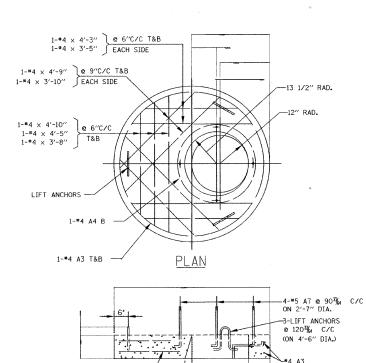
SECTION PRECAST TOP SLAB DETAIL SCALE: 3/4" = 1'-0'
