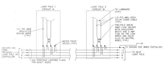
LIGHT POLE WIRING DETAIL
