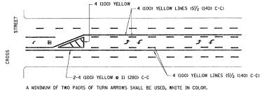
ADDITIONAL PAIRS SHALL BE PLACED AT 200' (60 m) TO 300' (90 m) INTERVALS.
