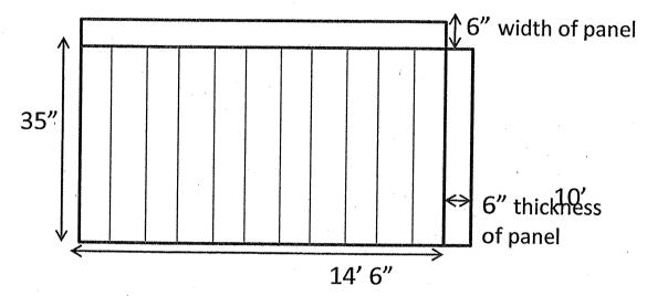
Wall is comprised of a series of panels, stacked on top. Wall height ranges from 12' to 17' in height. The beginning of the wall is stepped up to full 17' height in the middle.
