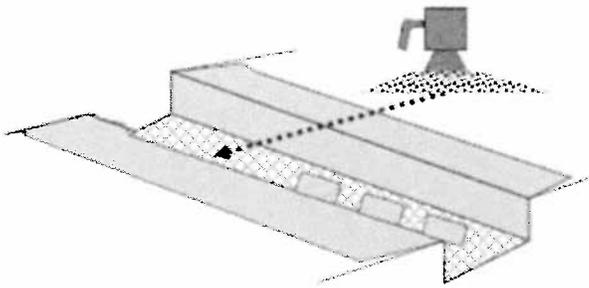
Step 5: Apply Silt Stop powder.
