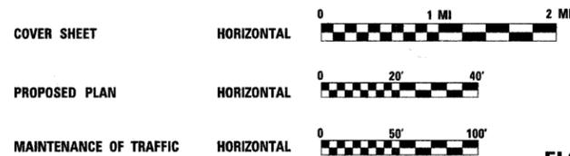
FULL SIZE PLANS HAVE BEEN PREPARED USING STANDARD ENGINEERING SCALES. REDUCED SIZED PLANS WILL NOT CONFORM TO STANDARD SCALES. IN MAKING MEASUREMENTS ON REDUCED PLANS, THE ABOVE SCALES MAY BE USED.
