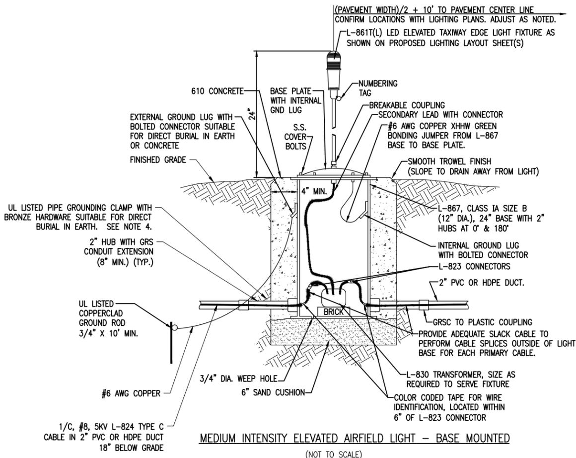
A LIGHT BASE GROUND SHALL BE INSTALLED AT EACH STAKE MOUNTED LIGHT AND EACH TRANSFORMER BASE/LIGHT CAN ASSOCIATED WITH RUNWAY LIGHTS, TAXIWAY LIGHTS, RUNWAY DISTANCE REMAINING SIGNS, AND LIGHTED RUNWAY/TAXI GUIDANCE SIGNS. THE LIGHT BASE GROUND SHALL BE A #6 AWG BARE COPPER CONDUCTOR CONNECTED TO THE GROUND LUG ON THE RESPECTIVE L-867 TRANSFORMER BASE/LIGHT CAN OR MOUNTING STAKE AND A 3/4-INCH DIAMETER BY 10- FEET LONG (MINIMUM) UL LISTED COPPER CLAD GROUND ROD.
