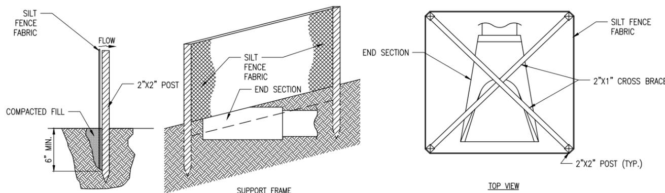
**FABRIC INLET/END SECTION PROTECTION**
