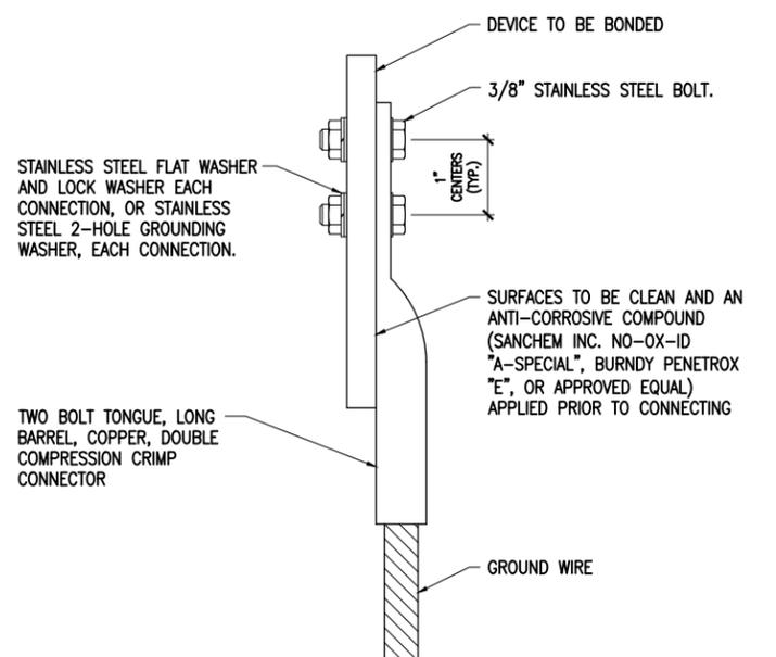
2 HOLE LONG BARREL COMPRESSION LUG TABLE (OR APPROVED EQUAL)
