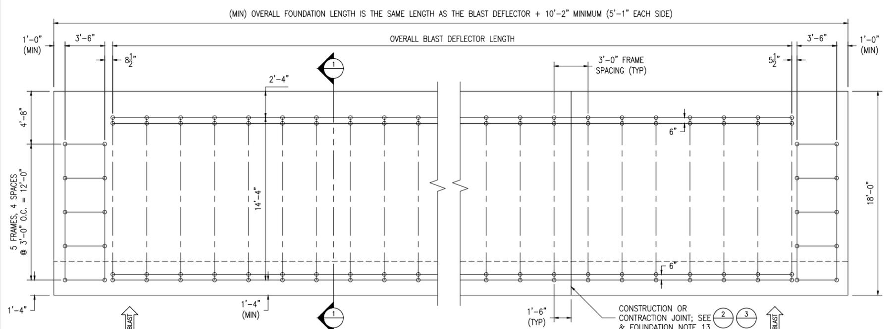
2 ANCHOR BOLT LAYOUT PLAN
