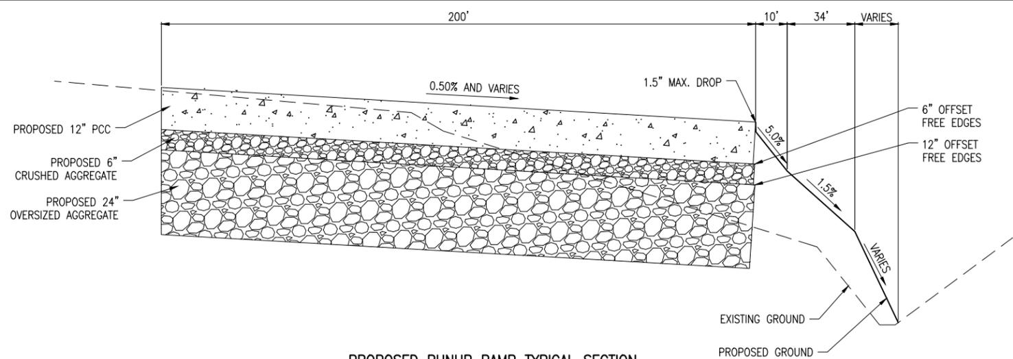
**PROPOSED RUNUP RAMP TYPICAL SECTION**
