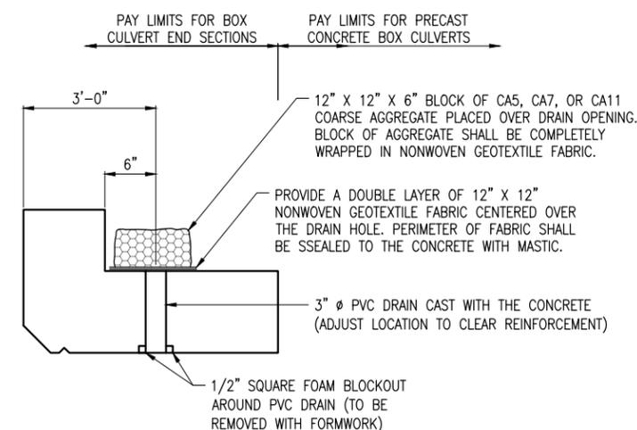
(ALL COSTS ASSOCIATED WITH FURNISHING AND CONSTRUCTING THE ABOVE DRAIN DETAIL WILL NOT BE MEASURED FOR PAYMENT BUT SHALL BE INCLUDED IN THE CONTRACT UNIT PRICE FOR THE ASSOCIATED WORK.)
