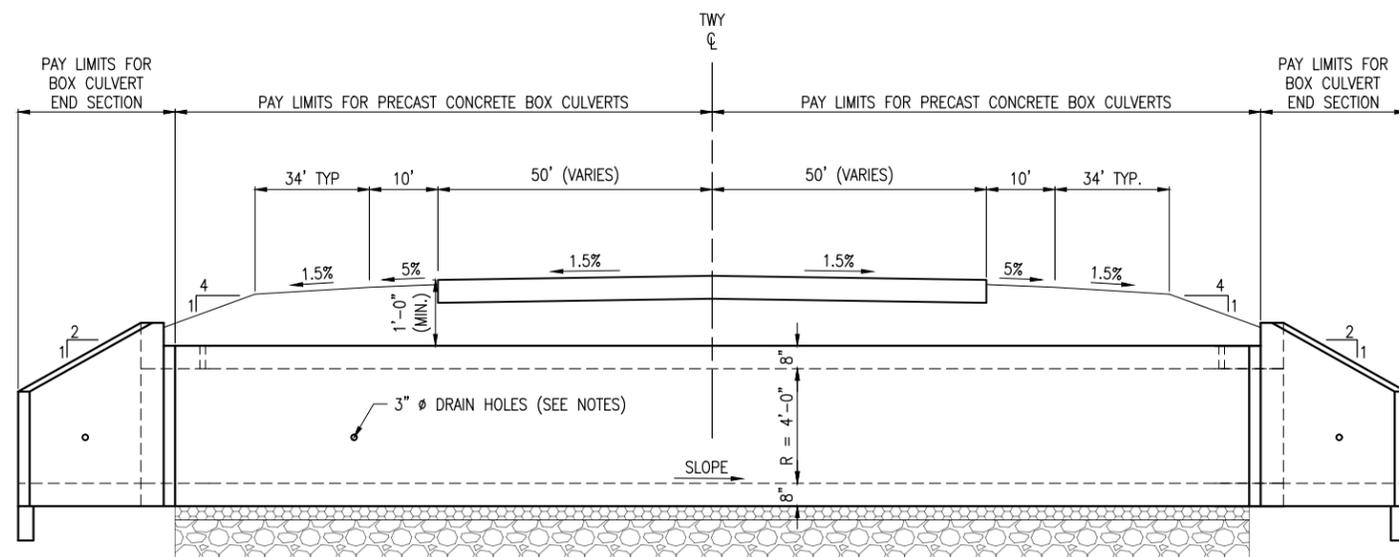
THE CONTRACTOR SHALL BE RESPONSIBLE FOR DETERMINING ALL DETAILS ASSOCIATED WITH THE PRECAST BOX CULVERT INCLUDING ANY STRENGTHENING OR STIFFENING PROVISIONS NECESSARY FOR HANDLING THE PRECAST SEGMENTS. CONCEPTUAL DETAILS FOLLOWED BY SHOP DRAWINGS AND DESIGN CALCULATIONS SEALED BY AN ILLINOIS LICENSED STRUCTURAL ENGINEER SHALL BE SUBMITTED TO THE ENGINEER FOR REVIEW AND APPROVAL.
