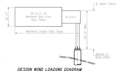
Parameters shown are basis for I.D.O.T. Standards Installations not within dimensional limits shown require special analysis for all components.
