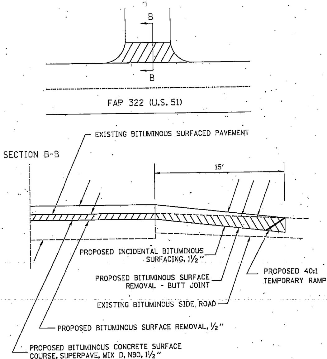
IF EXISTING BASE COURSE IS INADEQUATE, AS DETERMINED BY THE ENGINEER, THE SIDE ROADS SHALL BE CORED OUT AND AGGREGATE BASE COURSE, TYPE B SHALL BE PLACED FOR BASE. THE COST OF CORING OUT THE SIDE ROAD SHALL BE INCLUDED IN THE COST OF THE AGGREGATE BASE COURSE. IF EXISTING BASE COURSE IS DETERMINED TO BE ADEQUATE, THE AGGREGATE BASE COURSE SHALL BE DELETED AND THE PREPARATION OF THE BASE SHALL BE CONSTRUCTED ACCORDING TO ARTICLE 406.19.
