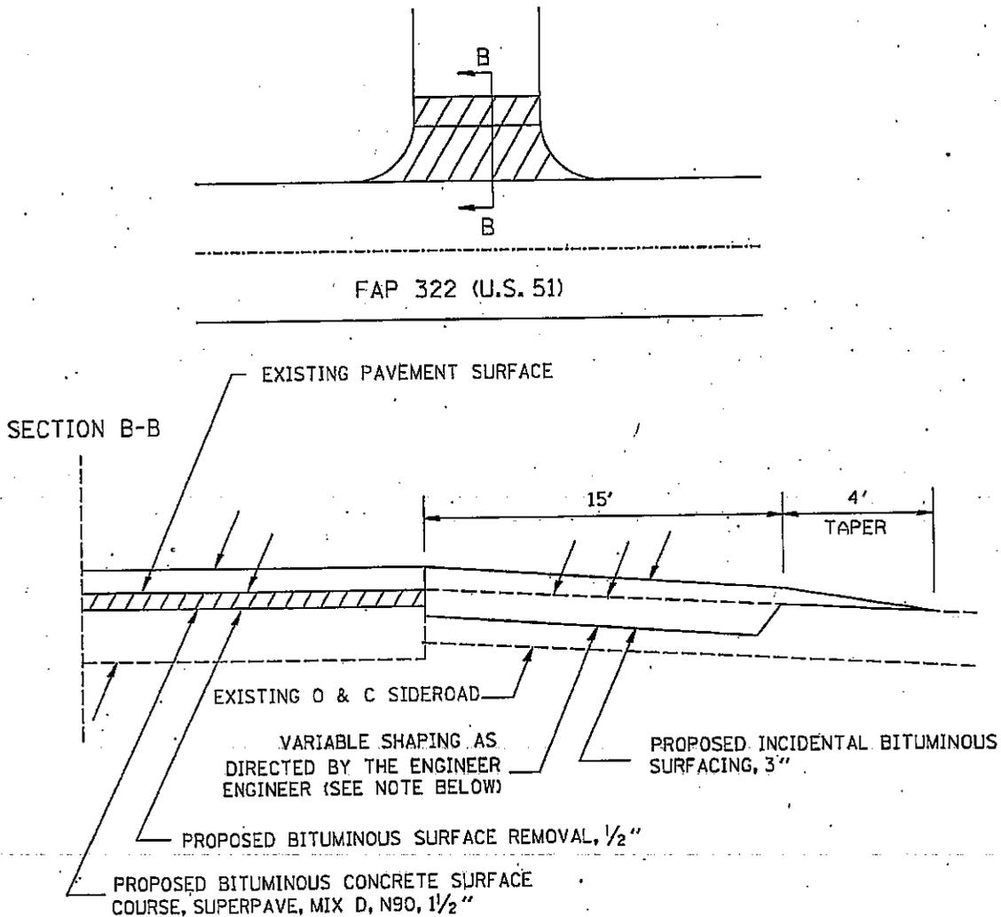
IF EXISTING SUB-BASE IS INADEQUATE; AS DETERMINED BY THE ENGINEER, THE SIDEROADS SHALL BE CORED OUT AND AGGREGATE SUB-BASE, TYPE B SHALL BE PLACED FOR BASE. THE COST OF CORING OUT THE SIDEROAD SHALL BE INCLUDED IN THE COST OF THE AGGREGATE BASE COURSE. IF EXISTING SUB-BASE IS DETERMINED TO BE ADEQUATE, THE AGGREGATE BASE COURSE SHALL BE DELETED AND THE PREPARATION OF THE BASE SHALL BE CONSTRUCTED ACCORDING TO ARTICLE 406.19
