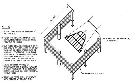
SILT FENCE PLACEMENT AT FLARED END SECTIONS (FES) OR HEADWALLS
