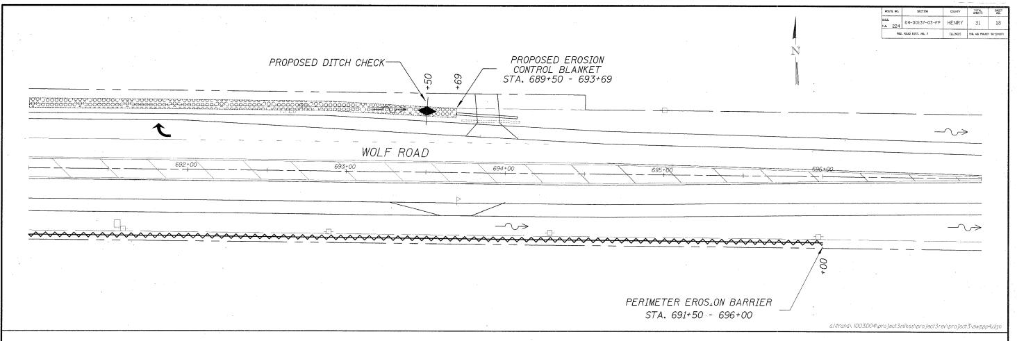
SEDIMENT COLLECTED DURING CONSTRUCTION OF THE VARIOUS TEMPORARY EROSION CONTROL SYSTEMS SHALL BE DISPOSED OF ON THE SITE ON A REGULAR BASIS AS DIRECTED BY THE ENGINEER. THE COST OF THIS MAINTENANCE SHALL BE INCLUDED IN THE UNIT BID PRICE FOR VARIOUS TEMPORARY EROSION CONTROL PAY ITEMS.
