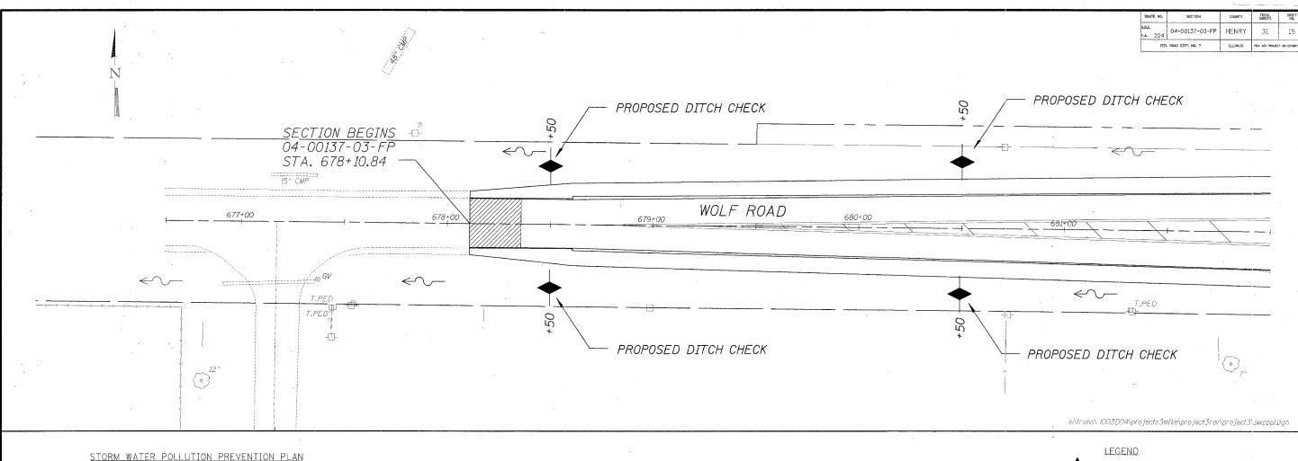
THE FOLLOWING PLAN IS ESTABLISHED AND INCORPORATED IN THE PROJECT TO DIRECT THE CONTRACTOR IN THE PLACEMENT OF TEMPORARY EROSION CONTROL SYSTEMS AND TO PROVIDE A STORM SEWER WATER POLLUTION PREVENTION PLAN FOR COMPLIANCE UNDER NPDES.
