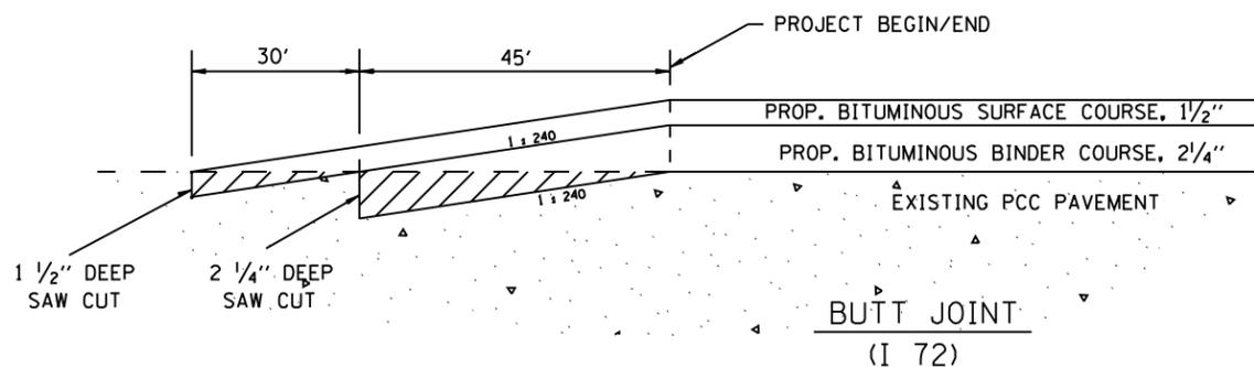
NOTE: TO BE PAID FOR AS PCC SURFACE REMOVAL - BUTT JOINT.
