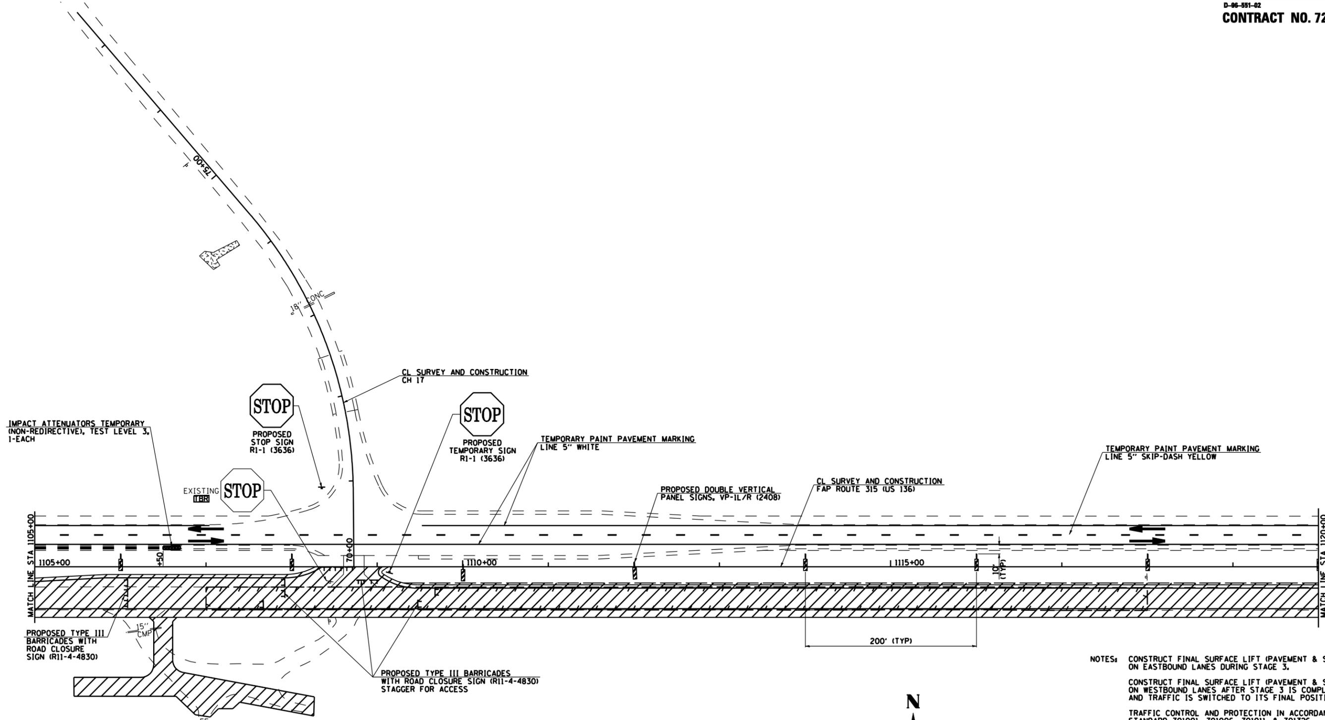
NOTES: CONSTRUCT FINAL SURFACE LIFT (PAVEMENT & SHOULDERS) ON EASTBOUND LANES DURING STAGE 3.
