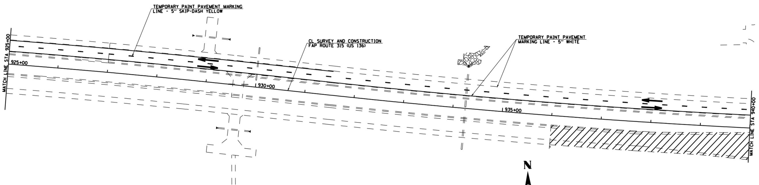
NOTES: CONSTRUCT FINAL SURFACE LIFT (PAVEMENT & SHOULDERS) ON EASTBOUND LANES DURING STAGE 3.
