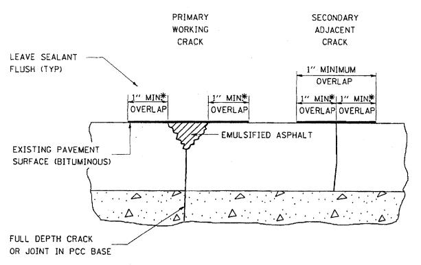
\*IN ALL LOCATIONS WHERE THE LONGITUDINAL CRACK CONFLICTS WITH EXISTING PAVEMENT MARKINGS (EITHER EDGE LINE OR LANE LINE) THE CRACK SHALL BE FILLED WITH EMULSIFIED ASPHALT. HOWEVER, THE 2" OVERLAP SHALL BE DELETED TO PREVENT UNNECESSARY DAMAGE TO THE EXISTING PAVEMENT MARKINGS. ALL EXCESSIVE DAMAGES TO EXISTING PAVEMENT MARKINGS & RAISED REFLECTIVE PAVEMENT MARKERS SHALL BE REPLACED AT THE EXPENSE OF THE CONTRACTOR.
