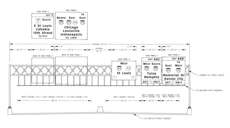
NOTE: THIS DETAIL IS NOT A TRUE CROSS SECTION OF THE ROADWAY BUT IS INTENDED TO SHOW THE PROPOSED PANEL LOCATIONS OVER THE ROADWAY LANES. SIGN PANELS SHOULD BE VERTICALLY CENTERED OVER LANES AND HORIZONTALLY CENTERED ON TRUSS IF POSSIBLE, OTHERWISE MAINTAIN 1.25' FROM BOTTOM OF SIGN PANEL TO WALKWAY.
