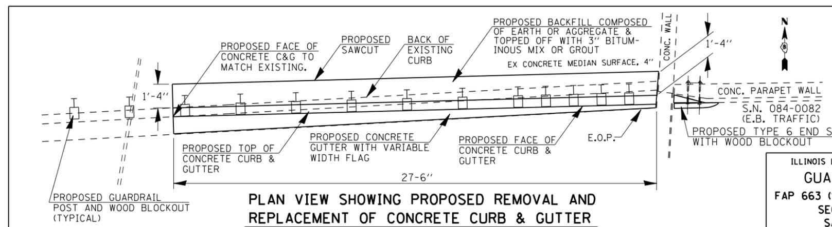
**PLAN VIEW SHOWING PROPOSED REMOVAL AND REPLACEMENT OF CONCRETE CURB & GUTTER
