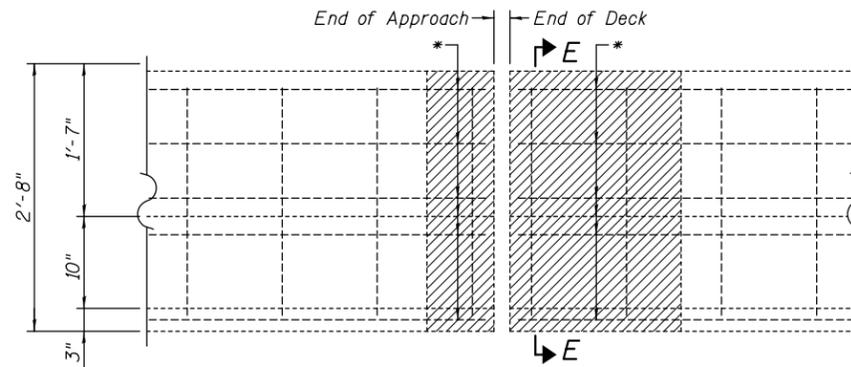
**ELEVATION AT CONCRETE MEDIAN**
