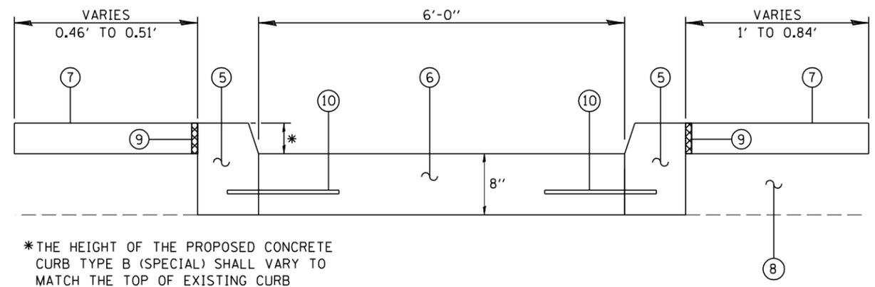
\*THE HEIGHT OF THE PROPOSED CONCRETE CURB TYPE B (SPECIAL) SHALL VARY TO MATCH THE TOP OF EXISTING CURB
