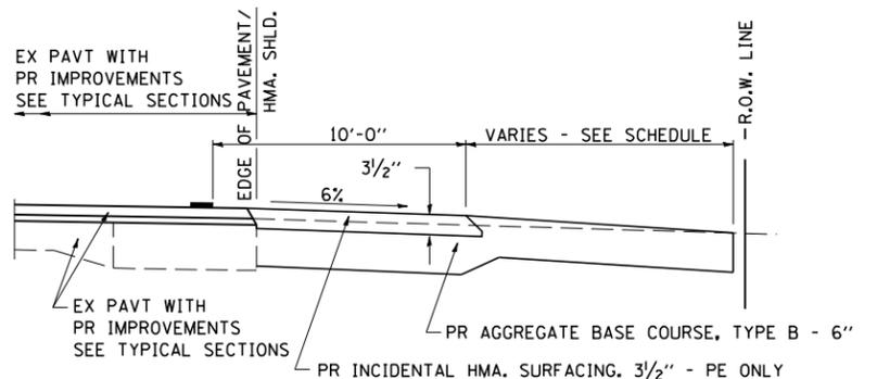
**SECTION A-A FOR EX EARTH/AGGREGATE FE & PE**
