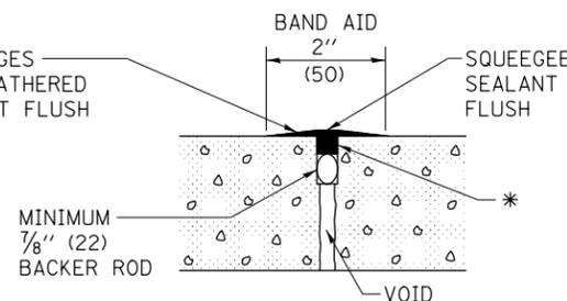
\* HOT ASPHALT CRACK SEALANT
