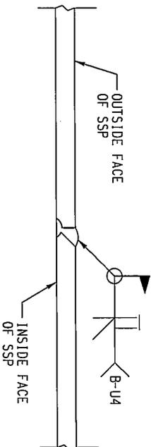
PIPE END WELD DETAIL
