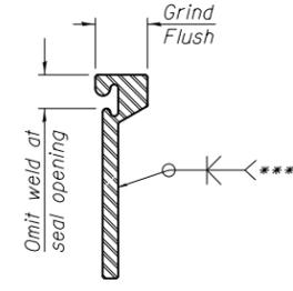
\*\*\* Back gouge not required if complete joint penetration is verified by mock-up.
