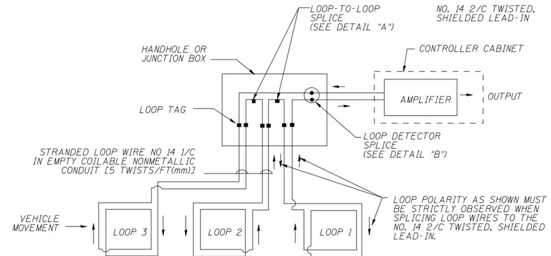
**DETECTOR LOOP WIRING SCHEMATIC**
