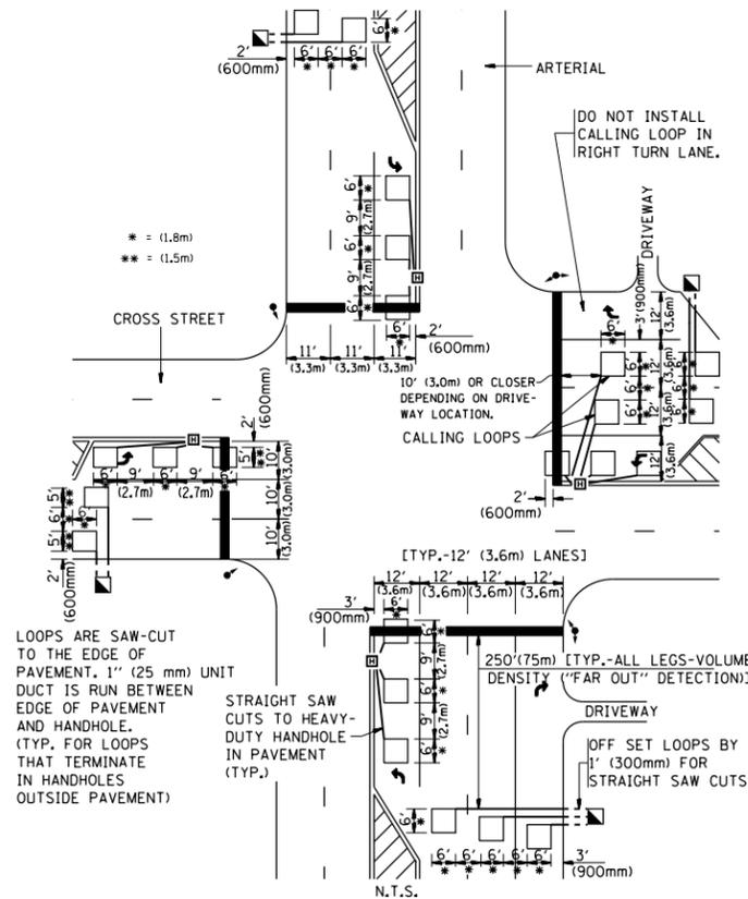
LOOPS ARE SAW-CUT TO THE EDGE OF PAVEMENT. 1" (25 mm) UNIT DUCT IS RUN BETWEEN EDGE OF PAVEMENT AND HANDHOLE. (TYP. FOR LOOPS THAT TERMINATE IN HANDHOLES OUTSIDE PAVEMENT)
