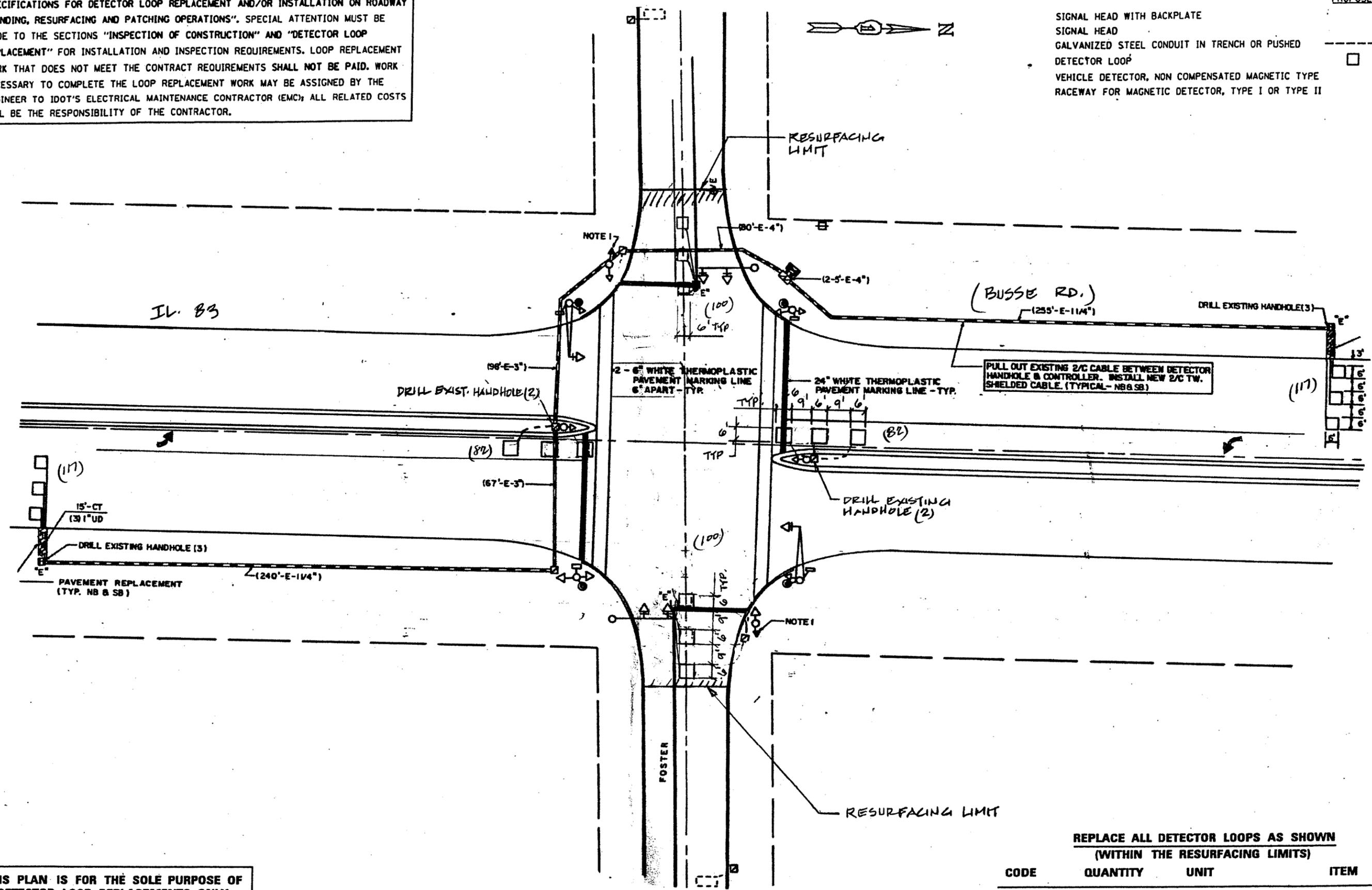
PULL OUT EXISTING 2/C CABLE BETWEEN DETECTOR HANDHOLE & CONTROLLER. INSTALL NEW 2/C TW. SHIELDED CABLE. (TYPICAL - NB & SB)
