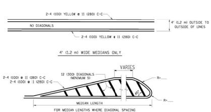
CANNOT BE ATTAINED, USE 5 (FIVE) EQUALLY SPACED
