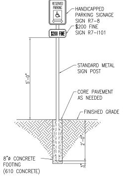
INTERNATIONAL SYMBOL OF ACCESSIBILITY - YELLOW PAINT; -PAID UNDER ITEM AR800571 "PAVEMENT MARKING -SPECIAL, HANDICAP SYMBOL" PER EACH - HANDICAPPED -CURB OR STRIPING SIGN (TYP) (SEE PLAN) 4" WIDE YELLOW -PAINT STRIPES **HANDICAP** TYPICAL 9'x20' (TYP.) PARKING DETAIL PARKING DETAIL NOT TO SCALE NOT TO SCALE
