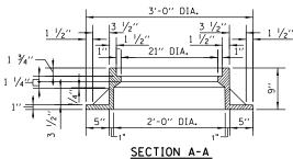
NOTE: METAL PLATES MUST BE FURNISHED FOR PERFORATED LIDS ON MANHOLES.
