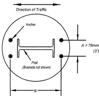
B (Bracket No. 1) = Depth of Post + 202mm (7-15/16")
