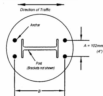
B (Bracket No. 1) = Depth of Post + 202mm (7-15/16")
