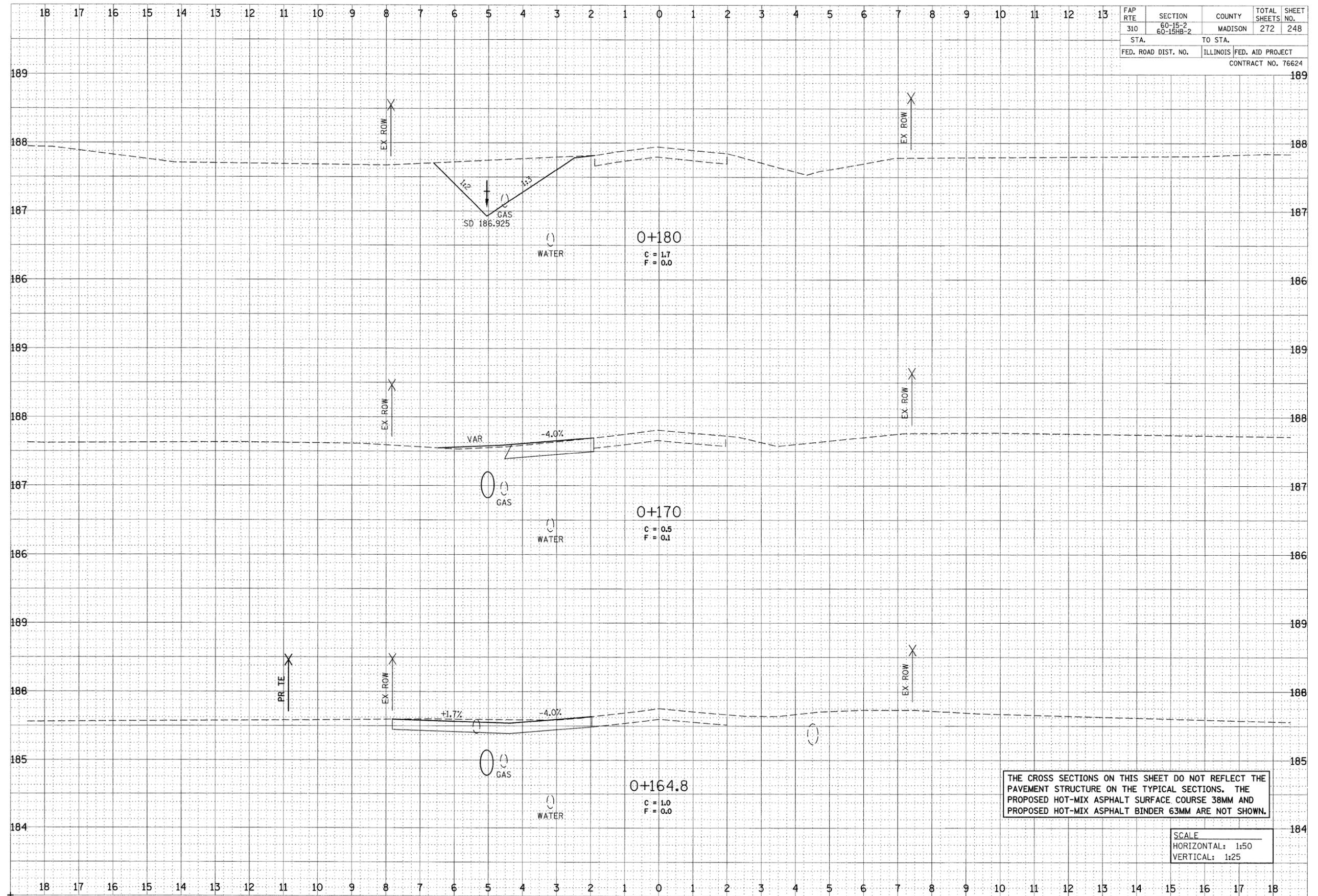
THE CROSS SECTIONS ON THIS SHEET DO NOT REFLECT THE PAVEMENT STRUCTURE ON THE TYPICAL SECTIONS. THE PROPOSED HOT-MIX ASPHALT SURFACE COURSE 38MM AND PROPOSED HOT-MIX ASPHALT BINDER 63MM ARE NOT SHOWN.
