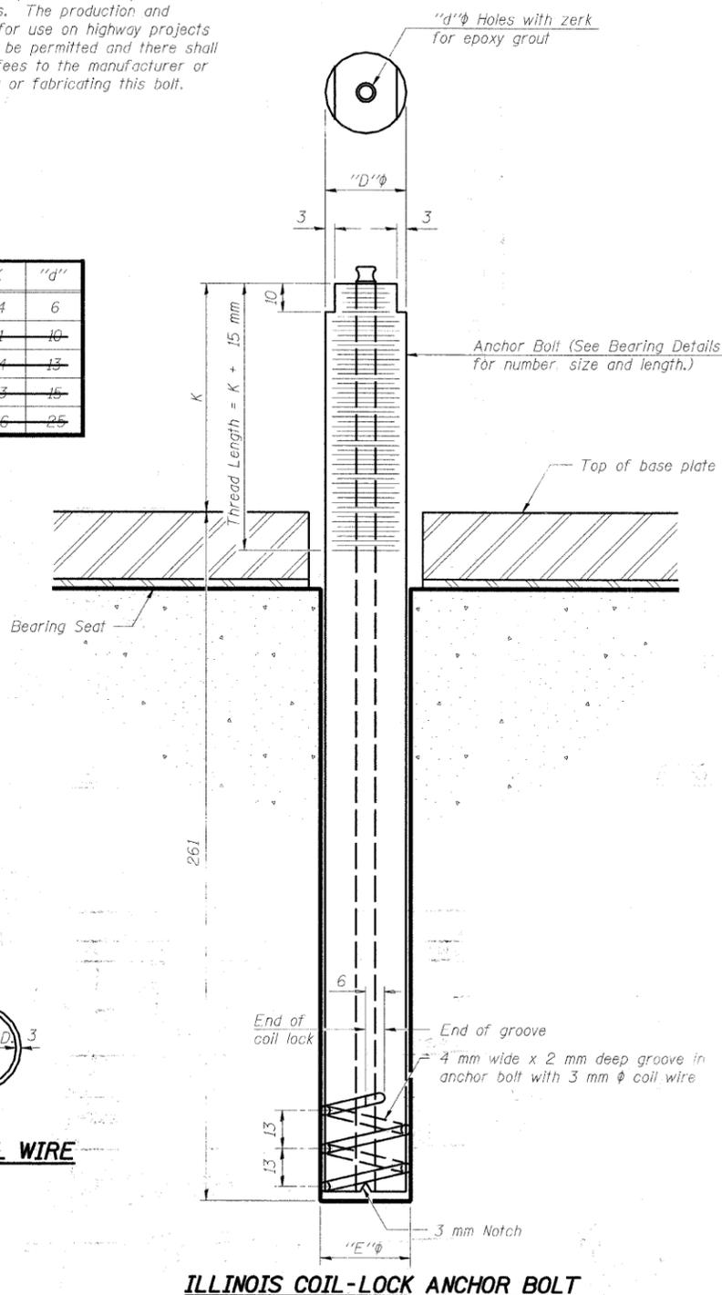
**MATERIALS FOR ILLINOIS COIL-LOCK ANCHOR BOLT**
