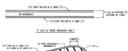
MEDIAN LENGTH FOR MEDIAN LENGTHS WHERE DIAGONAL SPACING CANNOT BE ATTAINED, USE 5 (FIVE) EQUALLY SPACED
