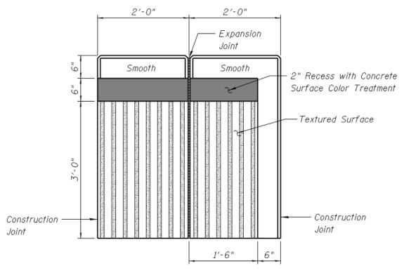
Include one horizontal and one vertical liner joint within textured surface.
