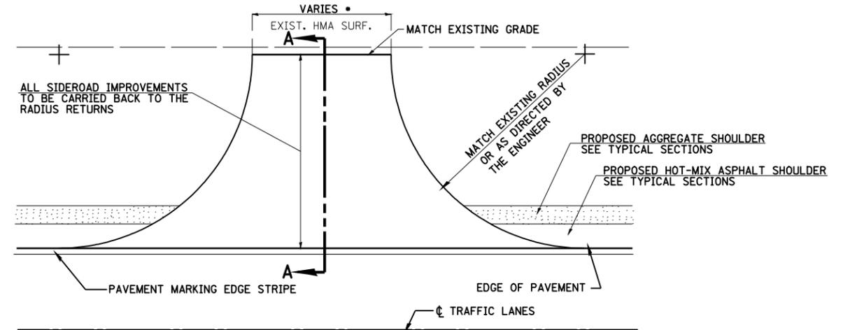
NOTES: THE REMOVAL OF EXISTING MATERIAL NECESSARY FOR SIDEROAD CONSTRUCTION WILL BE PAID FOR AS PREPARATION OF BASE.
