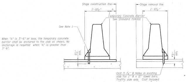
\* Dimension shown is minimum required embedment into concrete.
