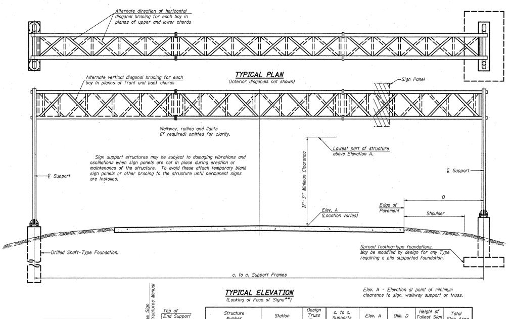
End Support 30 p.s.f. (See Sign Structures 10 p.s.f. Manual for max. sign areas) 31'-0". 'pe I-A Maximum Length c. to c. Support Frames (See Sign Structures Manual)
