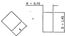
For diamond shaped sign with side S as shown, use required post size for a sign with W = 0.7S and D = 1.4S.
