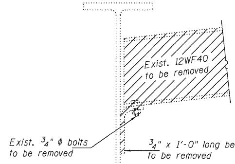
Exist. end diaphragms, bent P's, bolts and any existing welds shall be removed. Existing welds shall be removed using the air-arc method. Grind smooth all weld material remaining on the web. Cost included with Structural Steel Removal.
