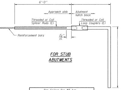
Bar Spiicer for #5 bar Min, Capacity = 23.0 kips - tension Min. Pull-out Strength = 12.3 kips - tension No. Required =
