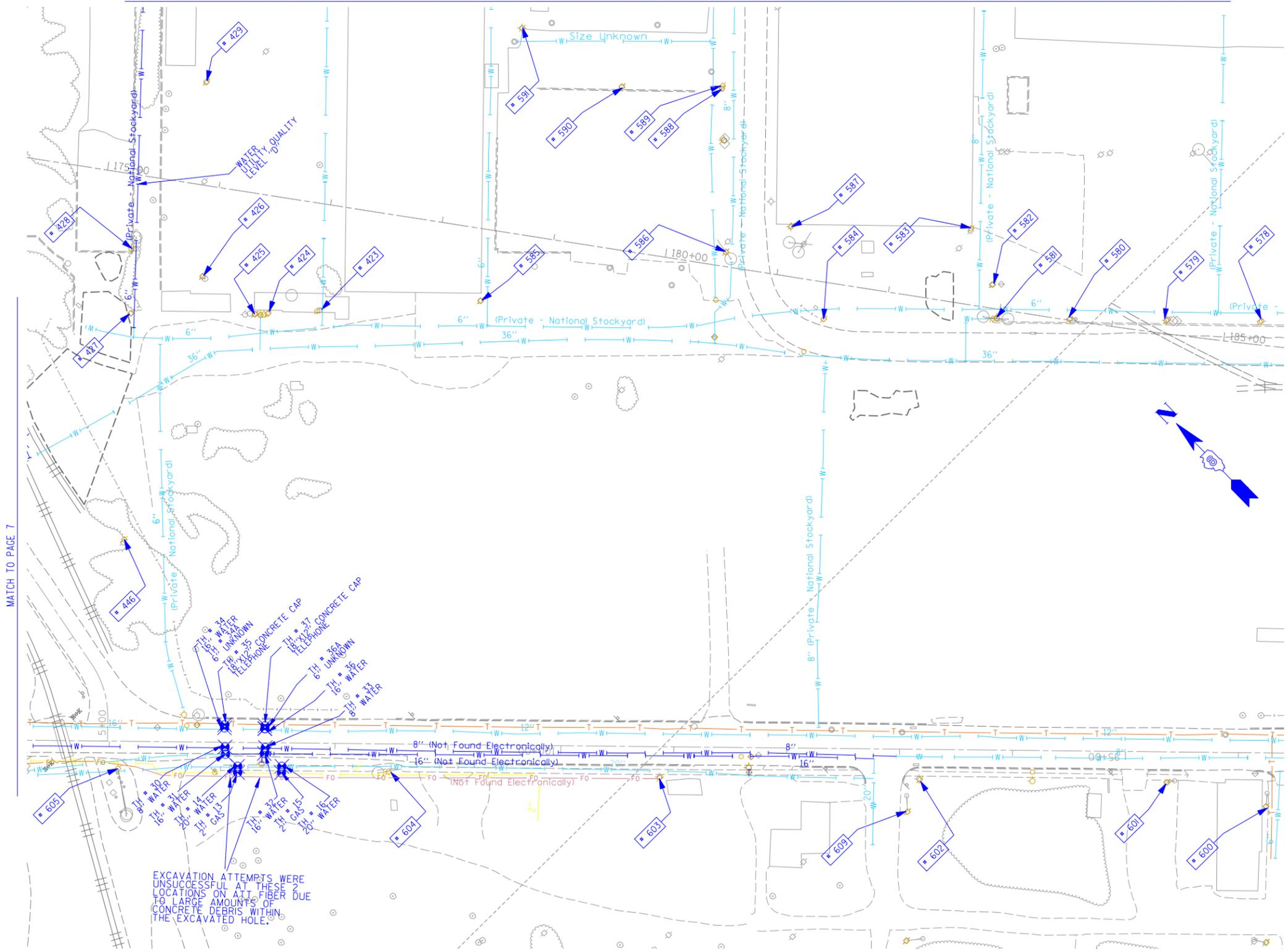
EXCAVATION ATTEMPTS WERE UNSUCCESSFUL AT THESE 2 LOCATIONS ON A11 FIBER DUE TO LARGE AMOUNTS OF CONCRETE DEBRIS WITHIN THE EXCAVATED HOLE.
