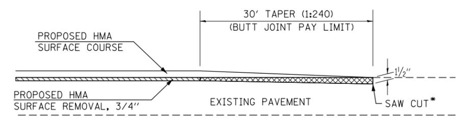
\* COST OF SAWCUT TO BE INCLUDED IN HOT-MIX ASPHALT SURFACE REMOVAL - BUTT JOINT
