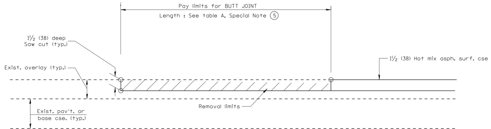
CASE 5 : WITH HOT MIX ASPHALT SURFACE REMOVAL (COLD MILLING)
