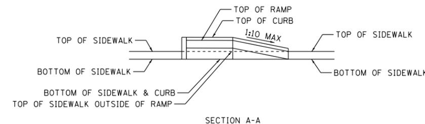
NOTE: SEE STATE HIGHWAY STANDARD 424011, CORNER PARALLEL CURB RAMP FOR SIDEWALKS FOR SIDE CURB DETAIL. THE CURB SHALL EXTEND A MINIMUM OF 2" ABOVE THE TOP OF RAMP.
