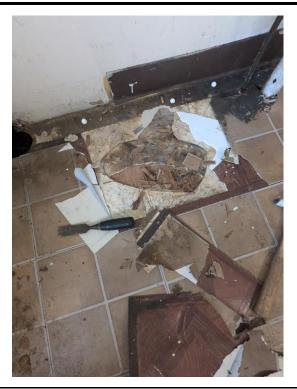
**Material Description:** White Linoleum (Under HA3 and HA-4) - Tested Positive for **Asbestos**
