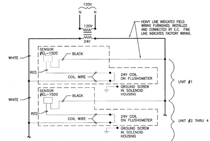
**C** FLUSH VALVE WIRING DIAGRAM
