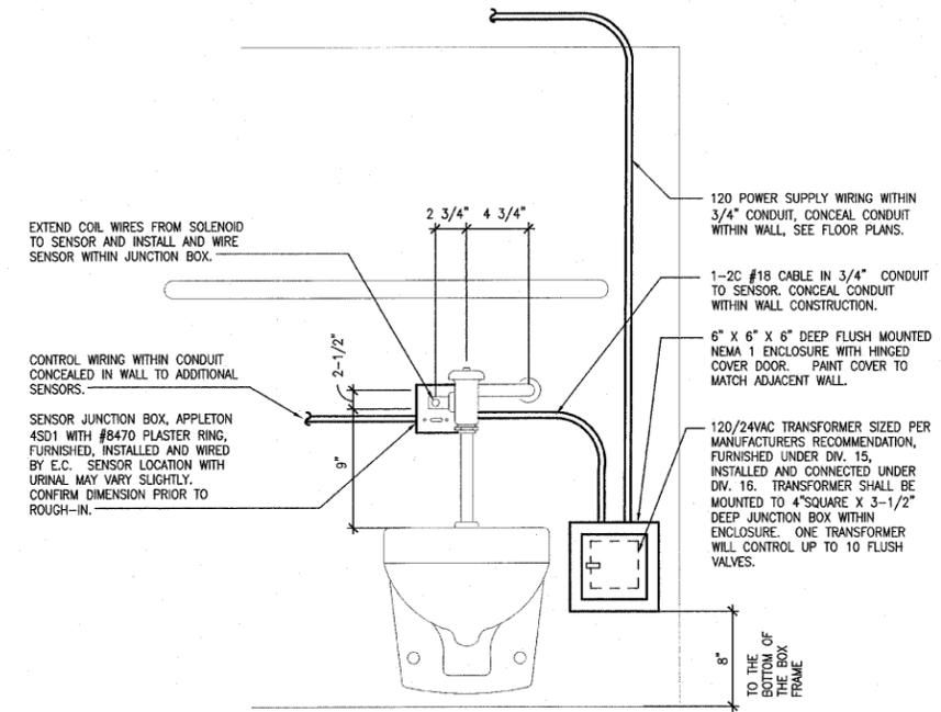
**B** FLUSH VALVE DETAIL FOR WATER CLOSETS AND URINALS
