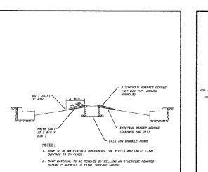
MANHOLE RAMPING DETAIL
