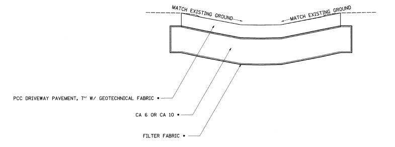
\* GEOTECHNICAL FABRIC, CA 6 OR CA 10, AND FILTER FABRIC ARE TO BE INCLUDED IN THE COST OF PCC DRIVEWAY PAVEMENT, 7"
