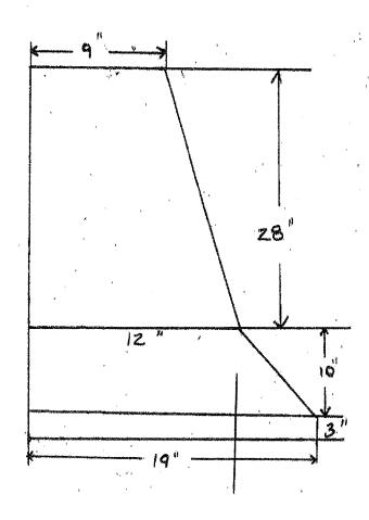
R & R 3' SECTION JUST PAST LIGHT POLE SHOULD DOWEL INTO CONCRETE SHOULDER.
