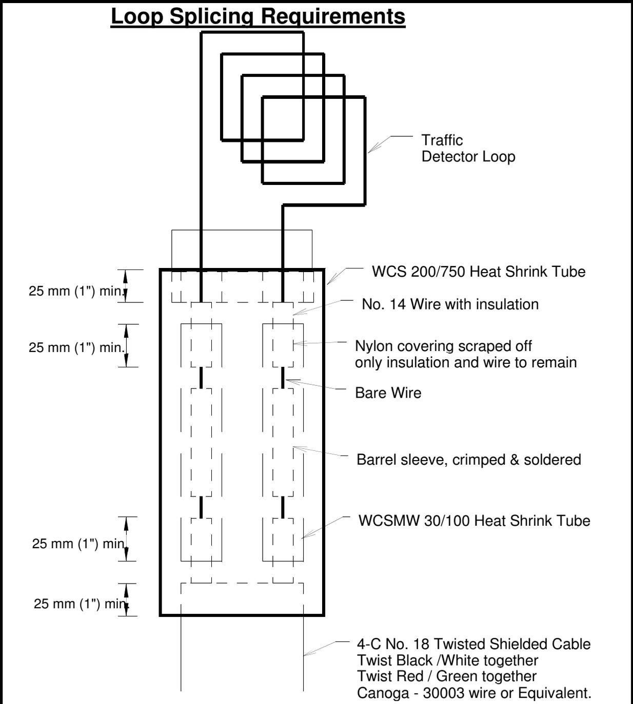
Minimum 25 mm (1") Heat Shrink Tube overlap on wire.
